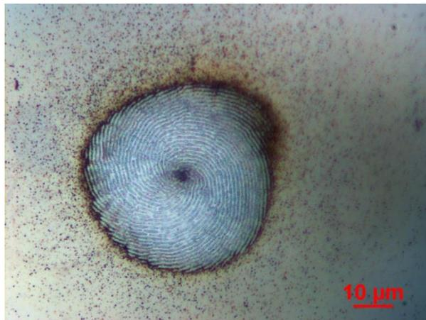
Fig.1 Spiral electric field micro-structuring on stainless steel
