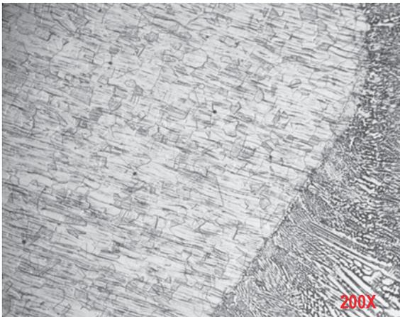
Fig. 8: HAZ of laser sample
