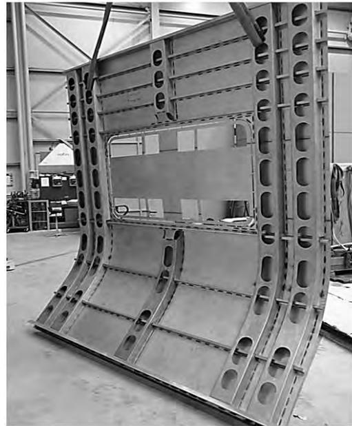
Fig. 5: LaserSeamStepper (picker) welded side panel of a passenger train
