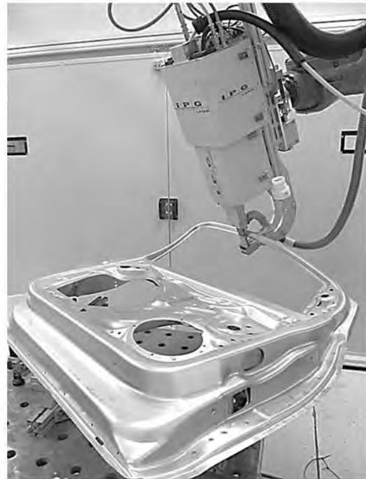
Fig. 3: Welding of 6mm flanges at door frame
