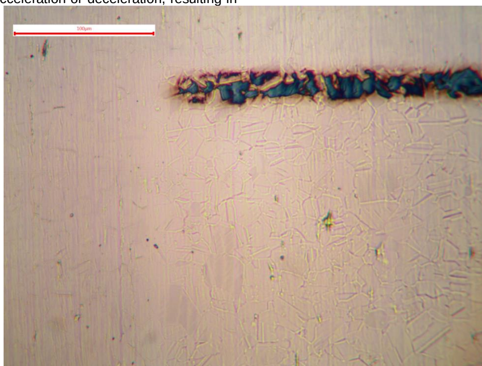
Figure 6 - The region where laser marking of the surface of the metal begins or ends with acceleration or deceleration resulting in larger surface energy densities. One can also notice the intentionally produced thin oxide film similar to that shown in Figure 4.
