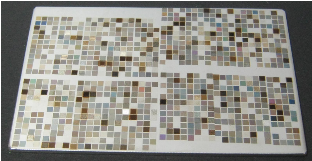
Figure 12 - 960 random unique colors of laser marking.
