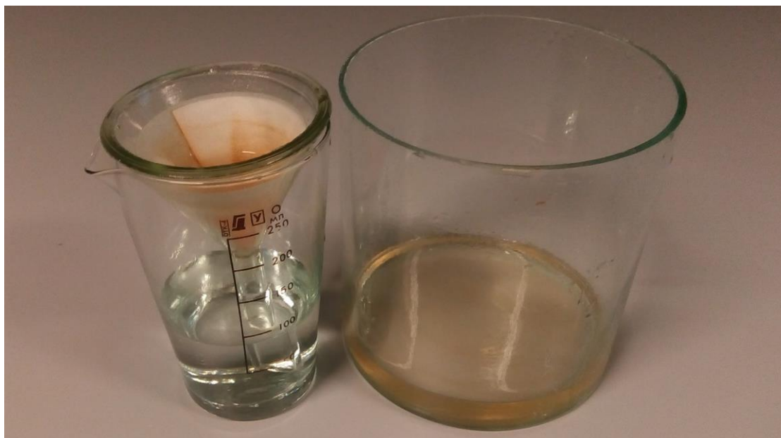
Figure 5 - The process of filtration of precipitate from a solution.
