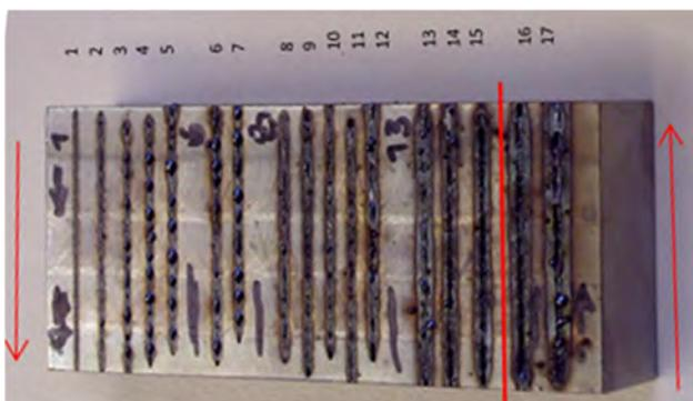
Bild 4: LB-Blindnaht; Spur1-7: 10m/min @  $P_L = 1-10$  kW, Spur 8-12: 5 m/min @  $P_L = 3, 5, 7, 9, 10$  kW, Spur 8-12: 2 m/min @  $P_L = 3, 5, 7, 9, 10$  kW
