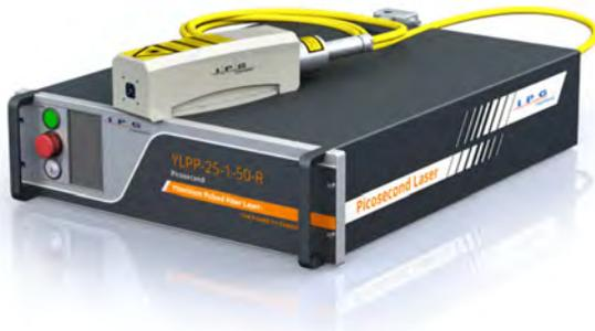
Image 1: The new ultrafast YLPP laser with 2-3ps pulse duration, 25 $\mu$ J pulse energy and 50 W average power.
