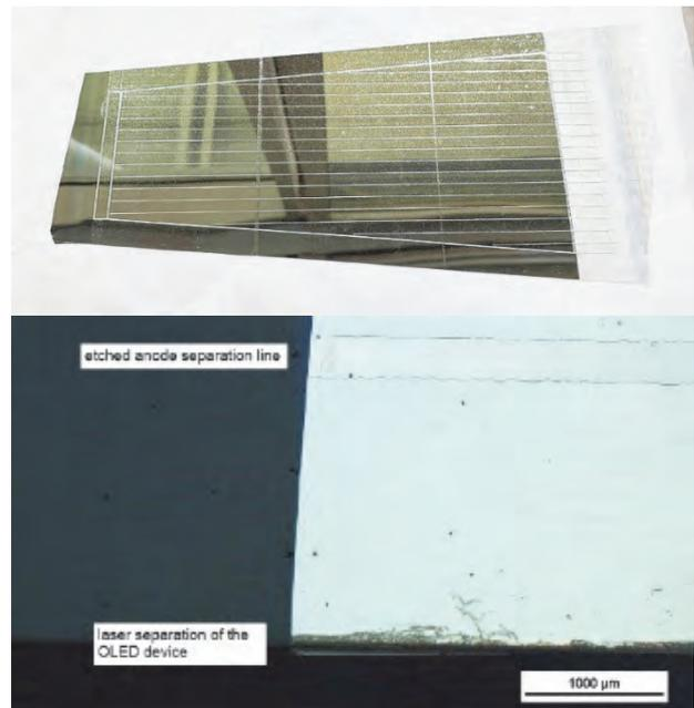
Fig. 1. Laser cut OLED-lighting device, full cutting of glass-OLED-glass stack
