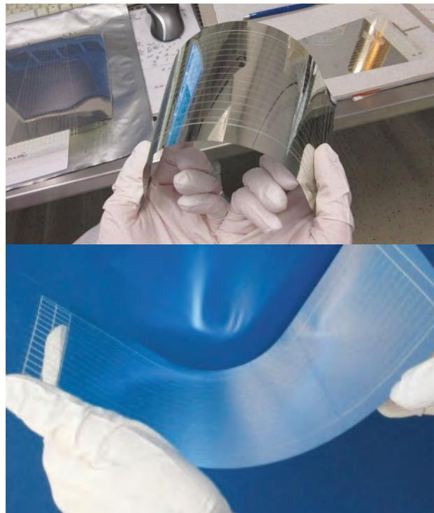
Fig. 4. Evaluation of behavior of laser cut OLEDs by manual bending and torsion tests
