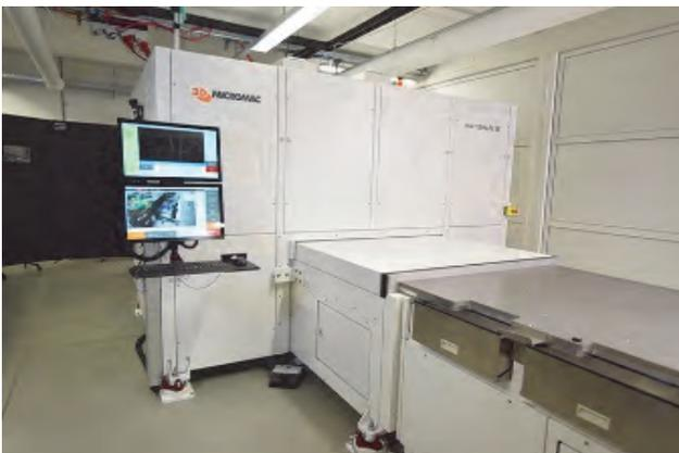
Fig. 6: Example of Laser System microSHAPE SE, dedicated for manual loading or line integration in sheet-to-sheet or roll-to sheet process flows
